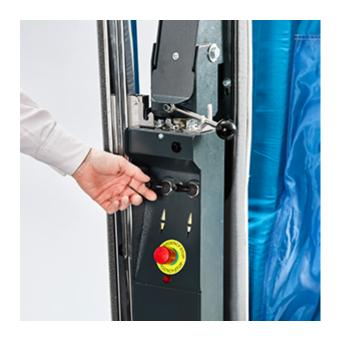
Pneumatic adjustment of sleeve clamps height
